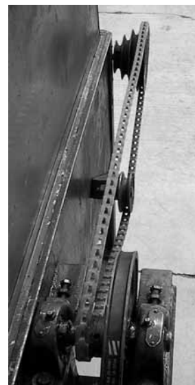
A view of the adjustable links (above) and the belt on the saw (below). Pictures by Jerry Sorensen.
